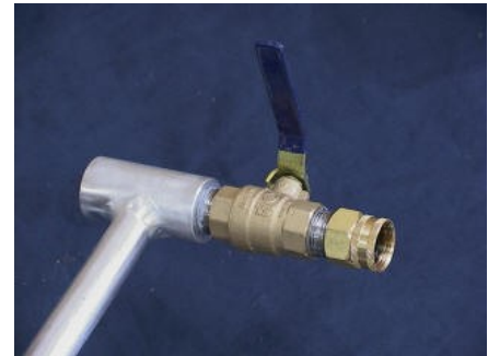
Valves on both the manifold and mud lances
